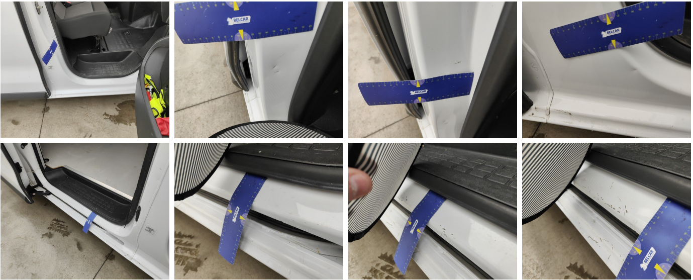
Rocker Panel Right // Smart Repair Medium-scratch + dent
