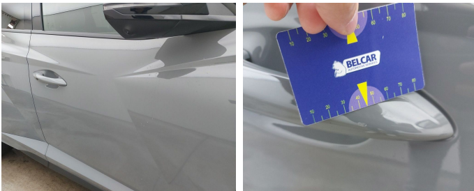
Door Front Right // Smart Repair Small-scratch
