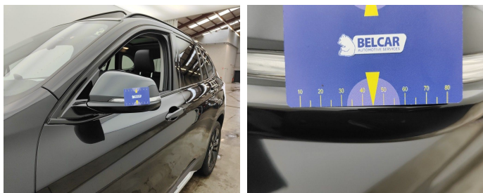
Side View Mirror Left // Replace & Painting-scratch
