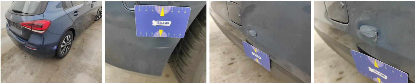
Bumper Rear // Replace & Painting-hole
