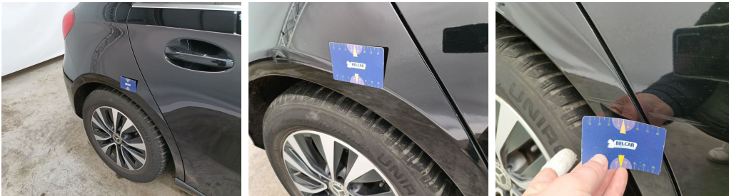
Wing Rear Right // Polish-scratch
