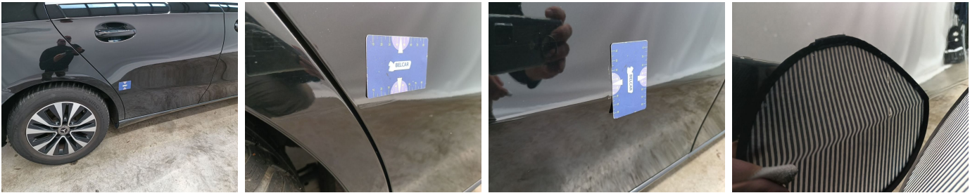
Door Rear Right // Repair & Painting-scratch + dent
