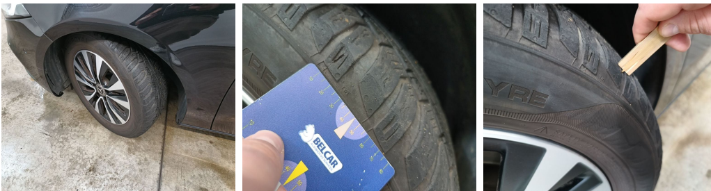
Tyre Front Left // Replace-worn
