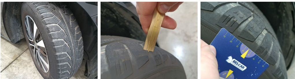
Tyre Front Right // Replace-worn
