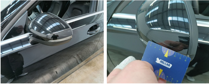
Side View Mirror Left // Polish-scratch
