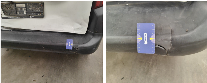
Bumper Rear // Replace without painting-cracked
