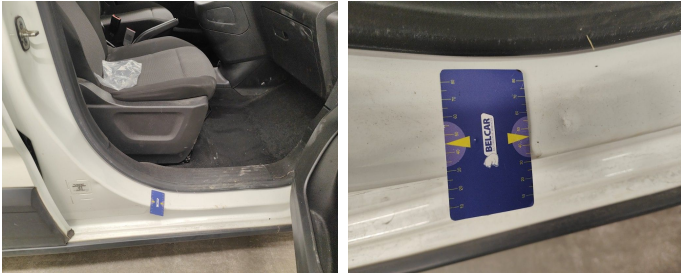
Rocker Panel Right // Smart Repair Medium-scratch + dent
