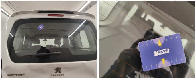
Rear Bonnet / Rear Window / Replace-scratch
