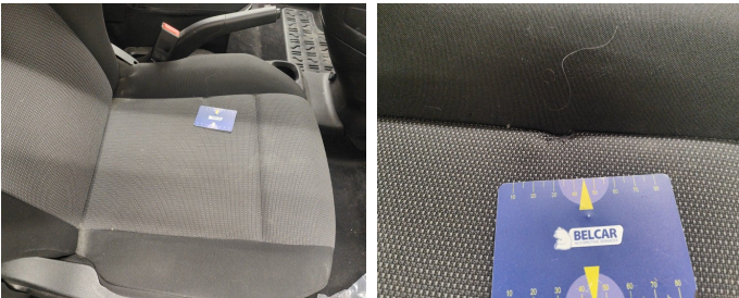
Seat Front Right / Bottom Coating / Replace-tear
