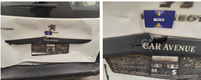
Rear Bonnet / Trim / Replace-cracked
