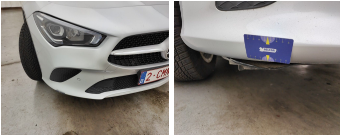
Wing Front right / Inner Fender / Replace-bad position
