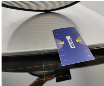
Bumper Front // Repair & Painting-scratch + dent
