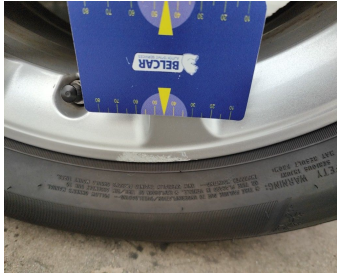
Wheel Alloy Front Left // Repair-scratch
