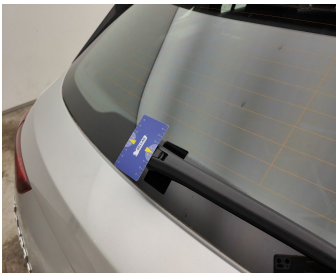
Back Side / Whiper Arm / Replace-cracked
