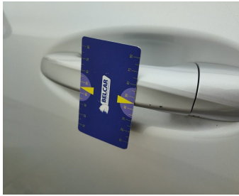
Door Front Left // Smart Repair Medium-scratch
