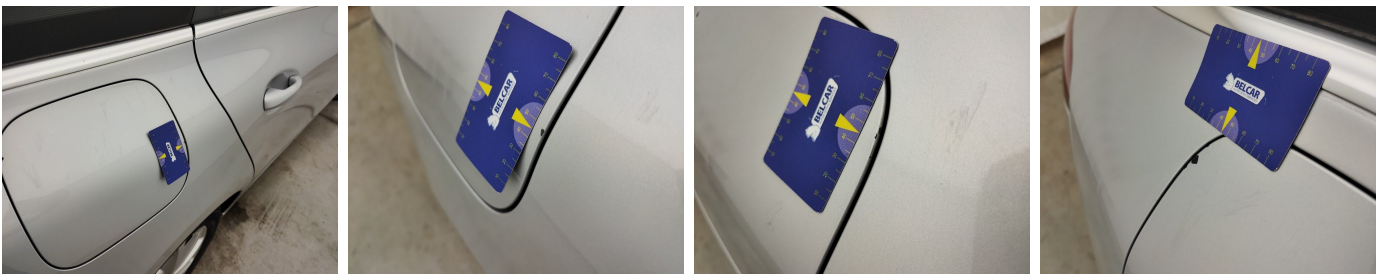
Wing Rear Right // Smart Repair Medium-stone chipping
