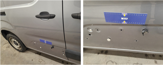
Door Rear Right / Trim / Replace-missing
