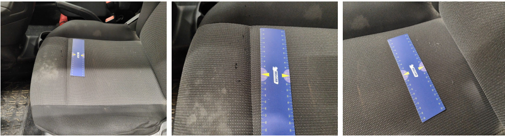
Seat Front Left / Bottom Coating / Replace-worn
