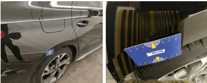
Wing Rear Right // Repair & Painting-scratch + dent
