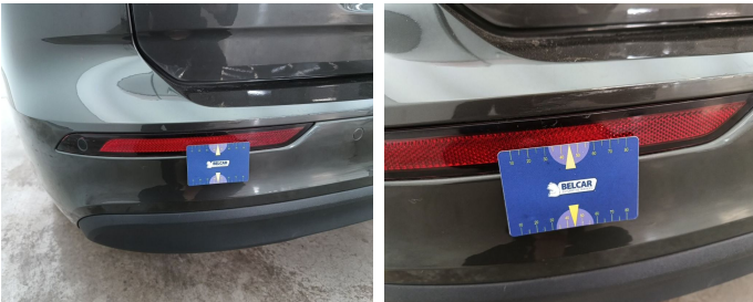
Back Side / Reflector L / Replace-scratch
