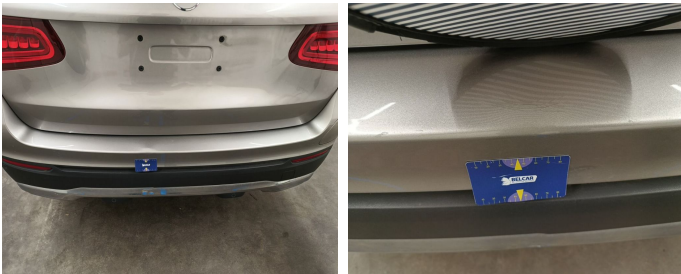
Bumper Rear // Repair & Painting-scratch + dent
