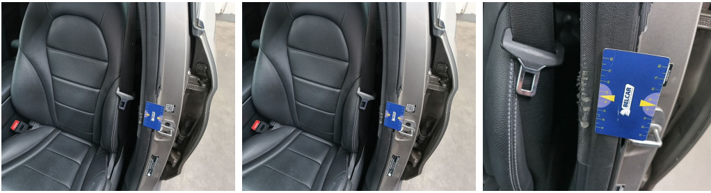
Interior / A Pillar Upper Cover / Replace-tear
