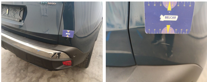
Bumper Rear // Smart Repair Medium-scratch
