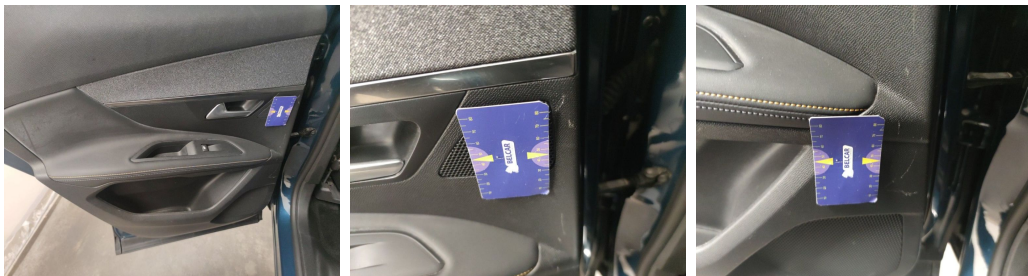
Rear Left Door Interior Coating // Replace Completely-scratch
