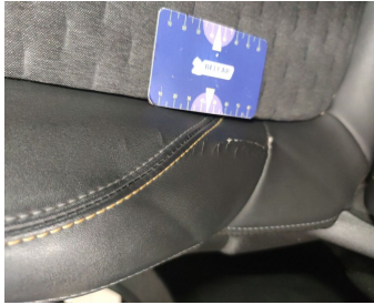
Seat Front Left / Bottom Coating / Replace-worn
