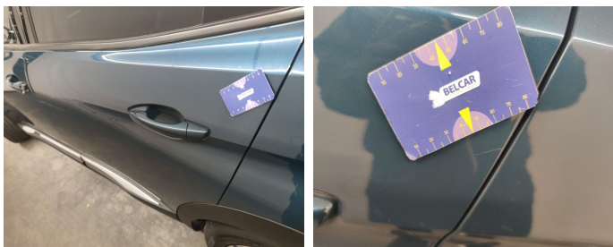
Door Rear Left // Smart Repair Medium-scratch
