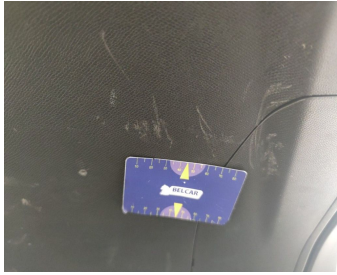
Trunk Lid Interior Coating / Complete Panel / Replace-scratch
