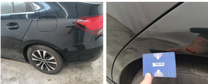
Wing Rear Left // Repair & Painting-bad repair
