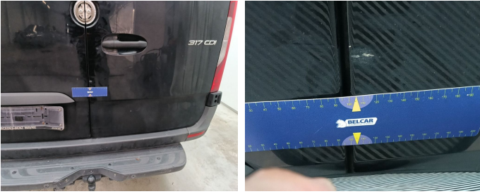
Rear Loading Door Right // Smart Repair Medium-scratch + dent
