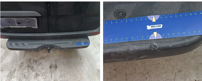
Bumper Rear / Spoiler / Replace-cracked
