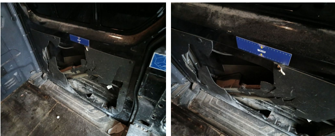
Trunk Lid Interior Coating / MDF Side Door Right / Replace-cracked
