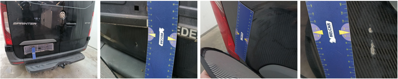
Rear Loading Door Left // Repair & Painting-scratch + dent
