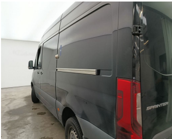
Wing Rear Left // Smart Repair Medium-dent
