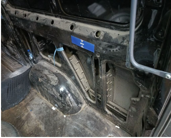
Trunk Compartment / Side Cover Right / Replace-missing
