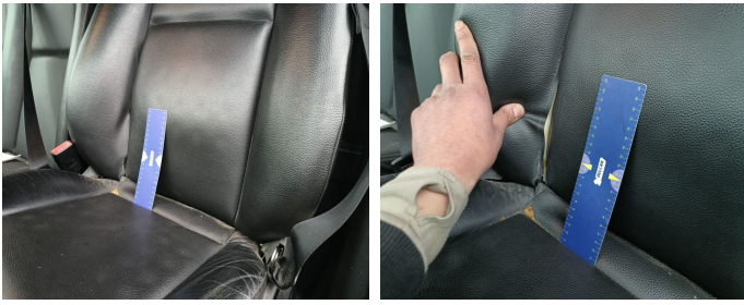
Seat Front Left / Rear Coating / Replace-cracked
