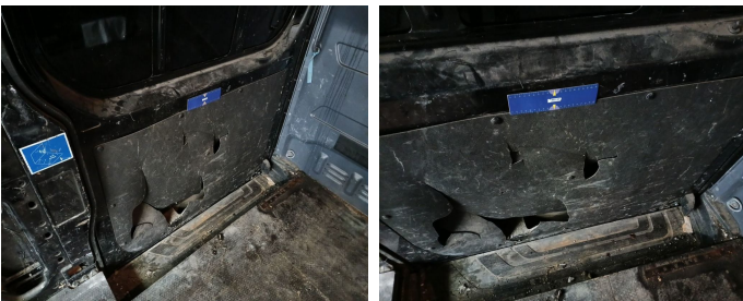
Trunk Lid Interior Coating / MDF Side Door Left / Replace-cracked
