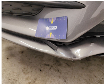
Bumper Front / Trim Right / Replace-cracked
