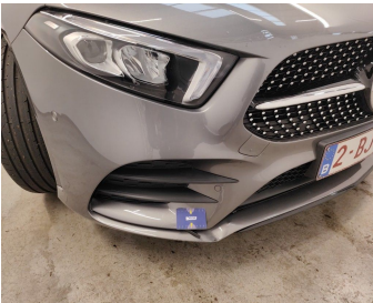
Bumper Front / Trim Right / Replace-cracked
