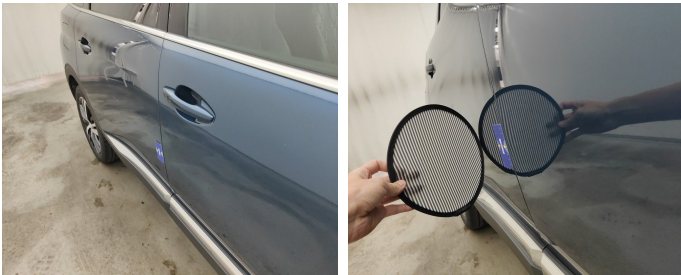
Door Front Right // Smart Repair Small-dent
