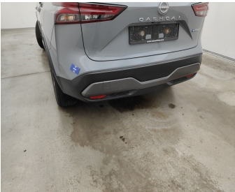
Bumper Rear / Trim Center / Replace-scratch
