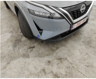
Bumper Front // Painting-stone chipping
