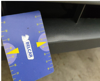
Bumper Front / Spoiler / Replace-dent
