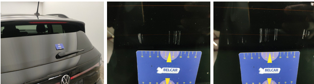
Rear Bonnet / Rear Window / Replace-scratch
