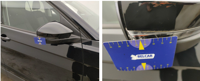
Side View Mirror Right / Direction Indicator / Replace-scratch
