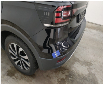
Bumper Rear // Painting-scratch
