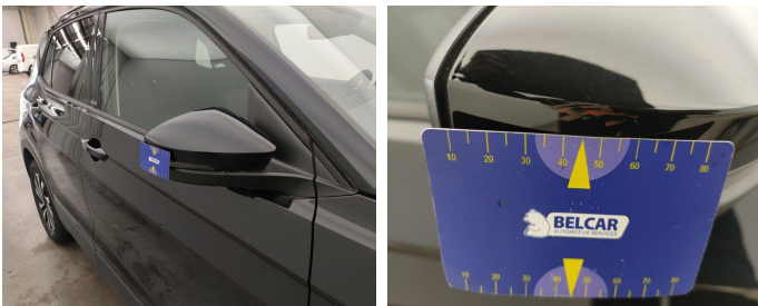
Side View Mirror Right // Painting-scratch
