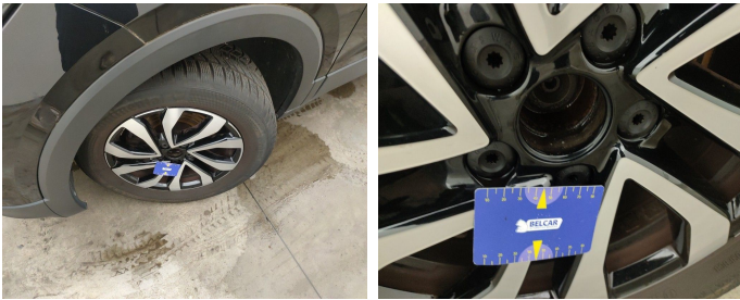
Wheel Front Left / Hub Cover With Logo / Replace-missing
