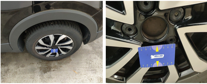
Wheel Rear Left / Hub Cover With Logo // Replace-missing
