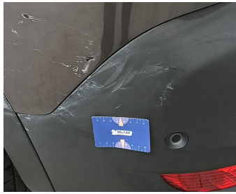
Bumper Rear / Lower Cover Not Painted / Replace-scratch
