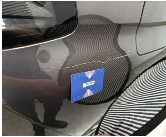
Wing Rear Right // Repair & Painting-scratch + dent
