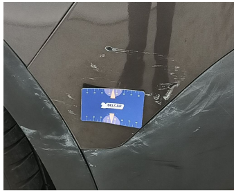
Bumper Rear // Smart Repair Large-scratch
