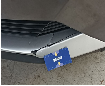
Bumper Front / Spoiler / Replace-cracked
