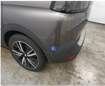
Bumper Rear // Smart Repair Large-scratch
