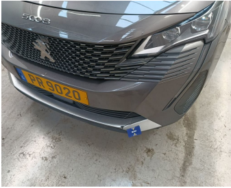
Bumper Front / Spoiler / Replace-cracked
