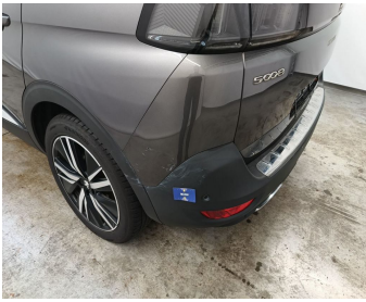
Bumper Rear / Lower Cover Not Painted / Replace-scratch
