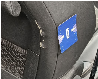
Seat Front Right / Rear Coating / Replace-tear
