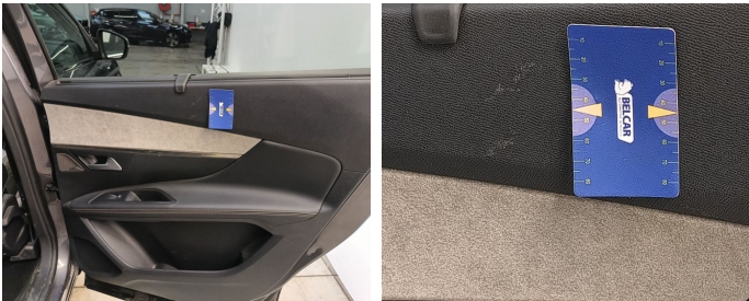
Rear Right Door Interior Coating // Replace Completely-scratch
