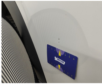
Door Rear Right // Repair & Painting-scratch + dent
