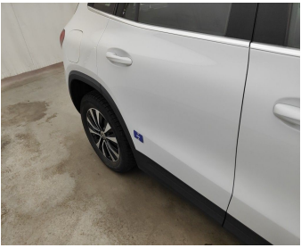
Door Rear Right // Repair & Painting-scratch + dent
