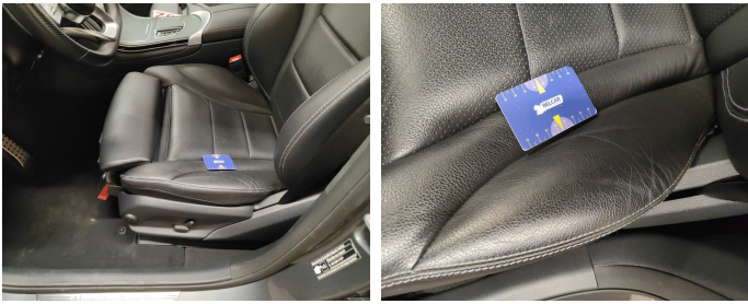
Seat Front Left / Bottom Coating / Replace-worn
