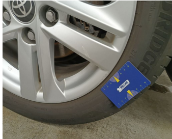
Wheel Alloy Rear Left // Repair-scratch
