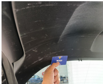
Trunk Lid Interior Coating / Complete Panel / Replace-scratch
