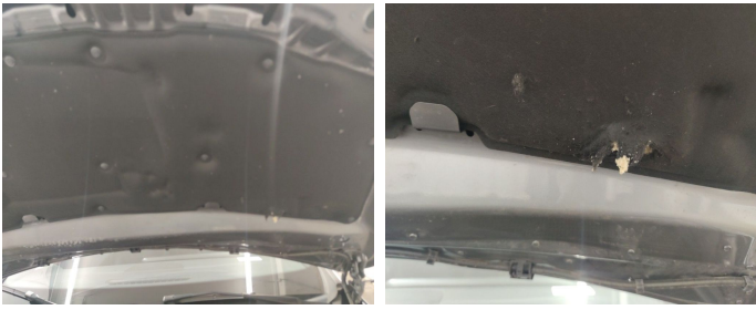
Front Bonnet / Insulation / Replace-hole
