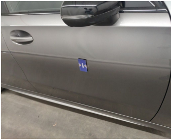
Door Front Right // Painting-scratch
