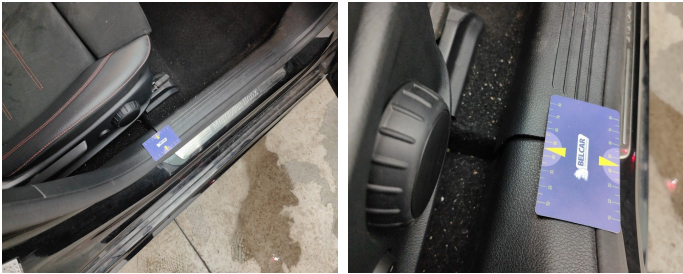
Interior / A Pillar Lower Cover / Replace-bad position
