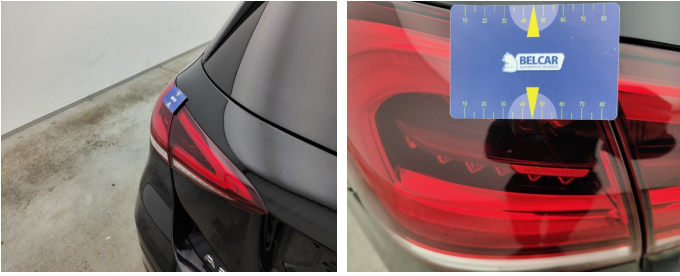
Light / Rear left / Replace-scratch
