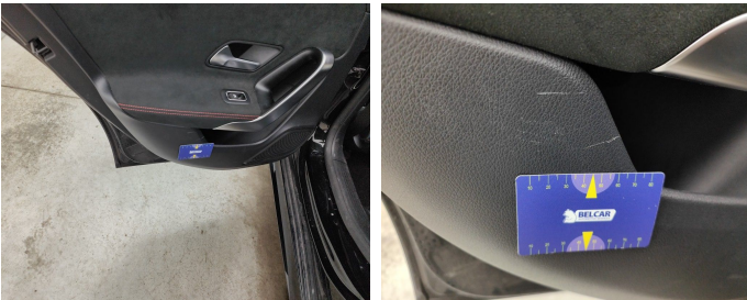
Rear Left Door Interior Coating // Replace Completely-scratch
