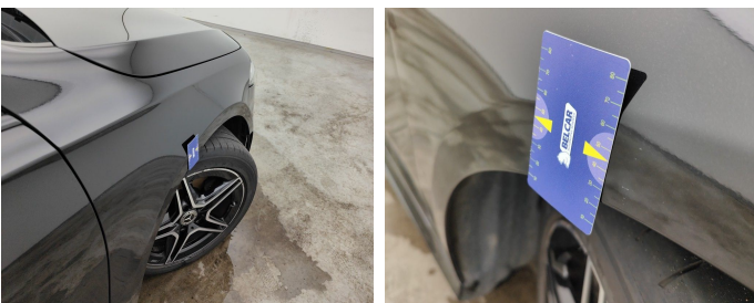
Wing Front right // Painting-scratch
