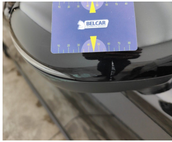
Side View Mirror Right // Painting-scratch
