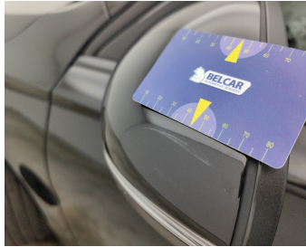
Side View Mirror Left // Painting-scratch
