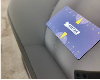
Bumper Front // Replace & Painting-cracked
