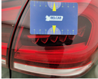
Light / Rear Right On Rear Bonnet / Replace-scratch
