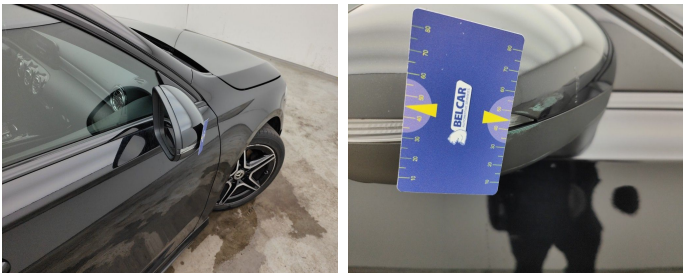
Side View Mirror Right / Direction Indicator / Replace-scratch
