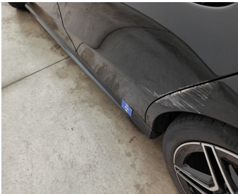
Rocker Panel Left // Painting-scratch
