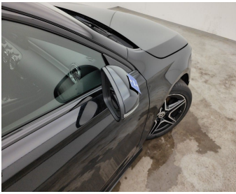
Side View Mirror Right // Painting-scratch
