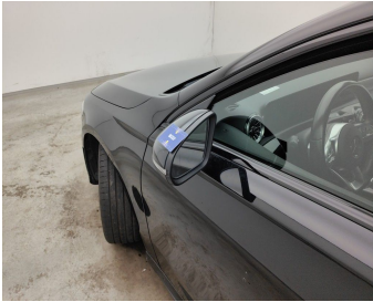
Side View Mirror Left // Painting-scratch
