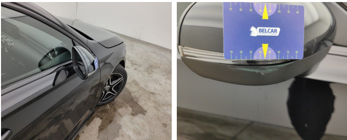
Side View Mirror Right // Replace Not Painted-scratch
