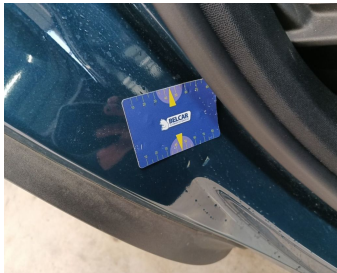
Rocker Panel Right // Smart Repair Medium-scratch + dent
