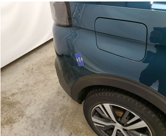
Wing Rear Right // Repair & Painting-scratch + dent
