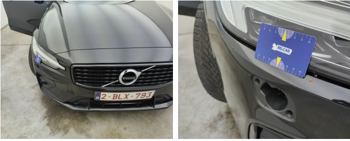
Front / Towing Cover / Replace-missing
