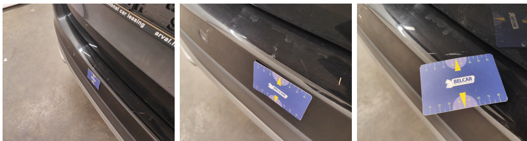
Bumper Rear // Painting-scratch
