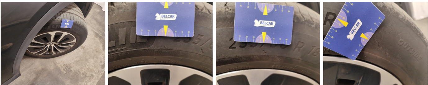
Tyre Front Right // Replace-tear
