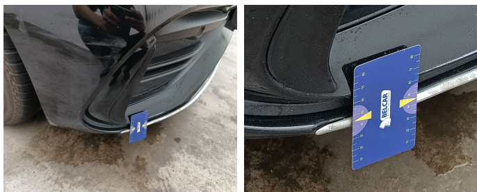
Bumper Front / Trim Right / Replace-cracked
