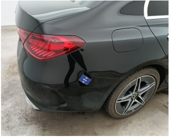
Bumper Rear // Painting-scratch
