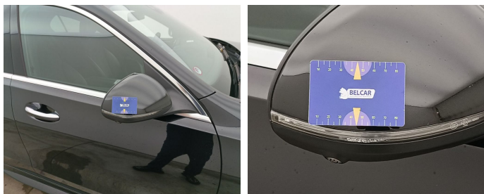
Side View Mirror Right / Direction Indicator / Replace-scratch
