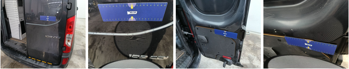
Rear Loading Door Right // Repair & Painting-dent
