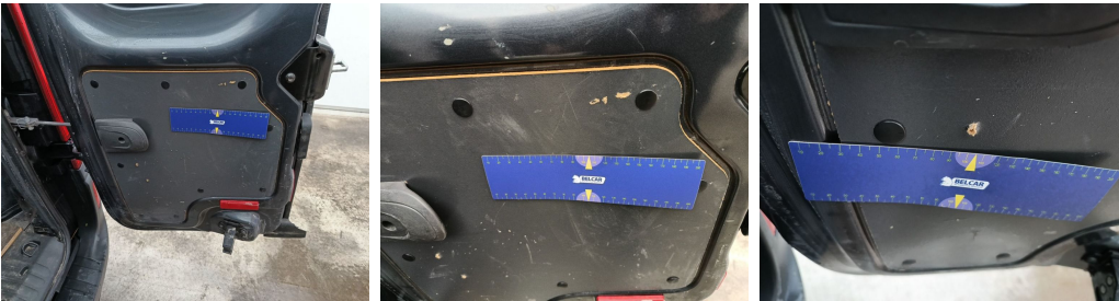
Trunk Compartment / Side Cover Right / Replace-cracked
