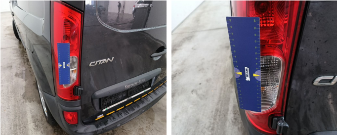
Light / Rear left / Replace-cracked
