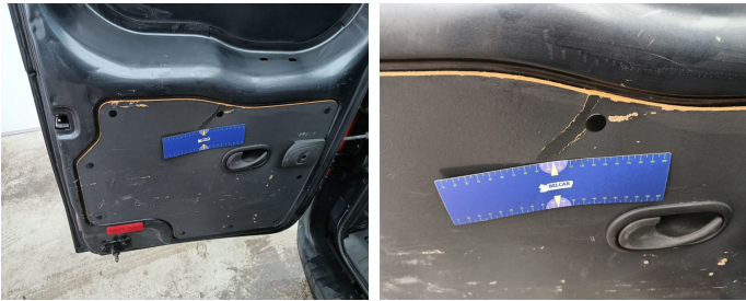
Trunk Compartment / Side Cover Left / Replace-cracked
