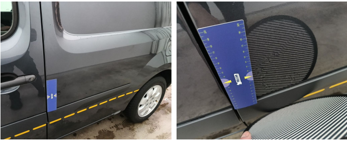
Wing Rear Left // Painting-bad repair
