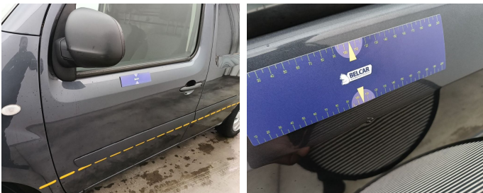
Door Front Left // Repair & Painting-scratch + dent
