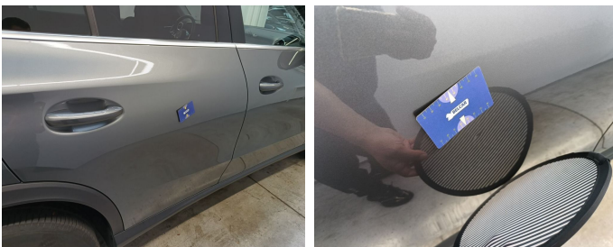
Door Rear Right // Smart Repair Small-dent
