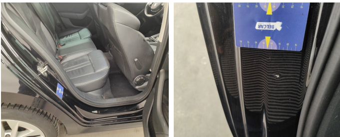
Rocker Panel Right // Smart Repair Medium-scratch + dent
