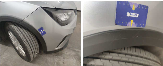
Bumper Front / Trim Right / Replace-scratch
