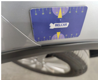
Wing Front Left / Trim / Replace-bad position
