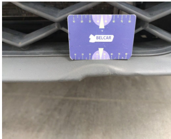
Bumper Front / Spoiler / Replace-dent
