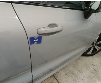
Door Front Right // Painting-scratch
