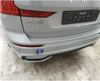
Bumper Rear // Painting-scratch
