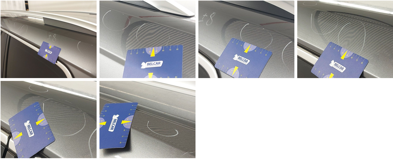
Roof // Smart Repair Medium-dent
