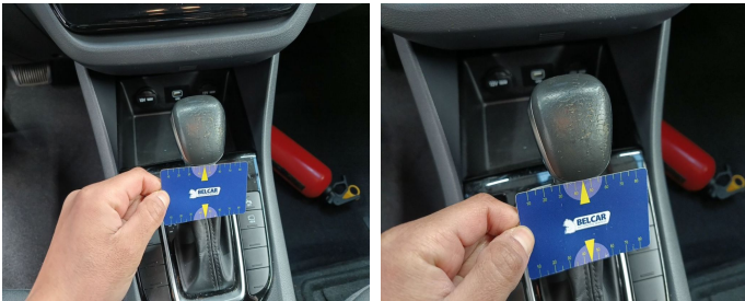
Central Console / Gear Lever / Replace-cracked
