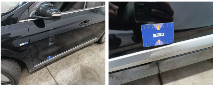
Door Front Left / Trim / Replace-scratch
