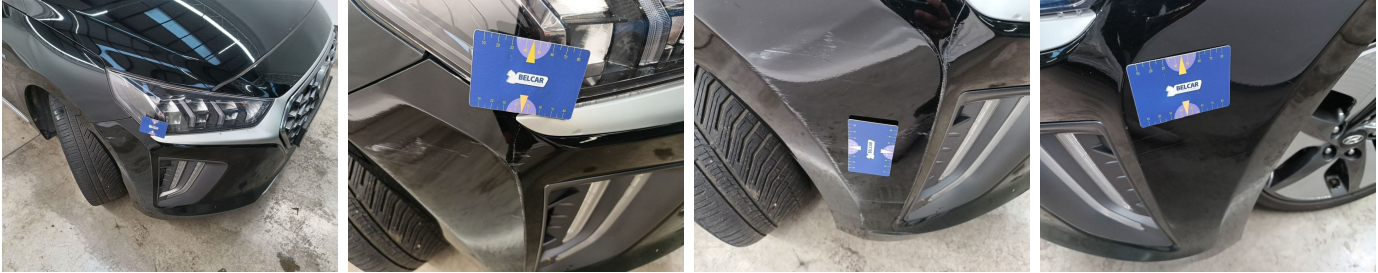
Bumper Front // Replace & Painting-cracked
