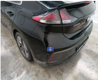
Bumper Rear // Painting-scratch
