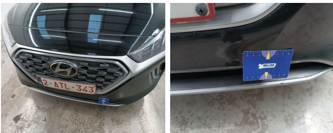
Bumper Front / Spoiler / Replace-scratch
