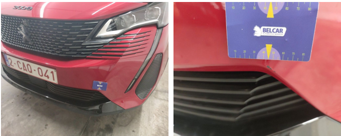
Bumper Front // Smart Repair Medium-scratch
