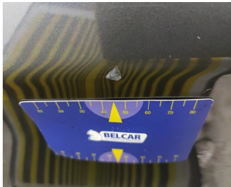
Door Rear Left // Painting-scratch + dent
