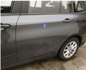
Door Rear Left // Painting-scratch + dent
