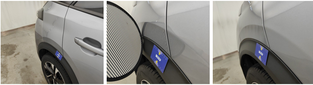
Wing Rear Right // Painting-bad repair
