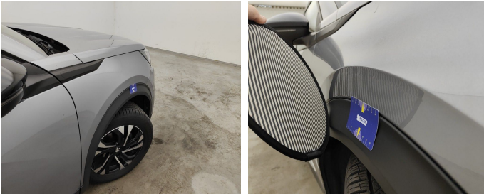
Wing Front right // Painting-bad repair
