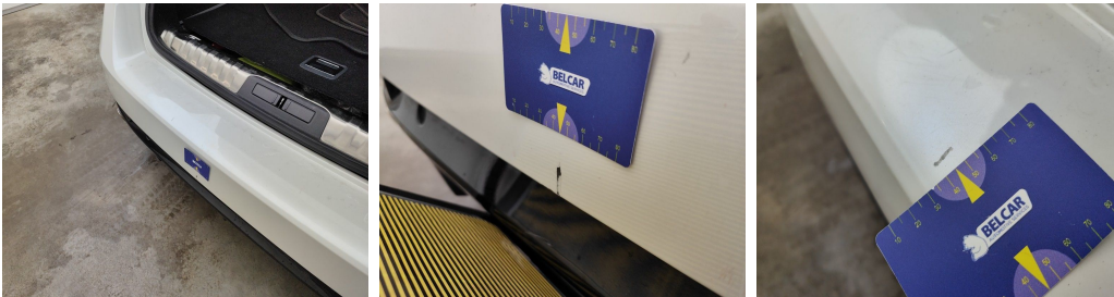
Bumper Rear // Repair & Painting-scratch + dent
