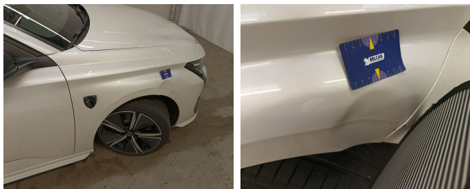
Wing Front right // Repair & Painting-scratch + dent
