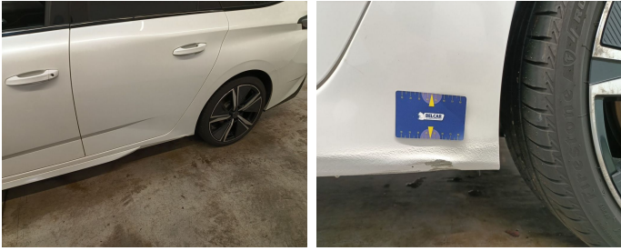
Rocker Panel Left // Repair & Painting-scratch + dent
