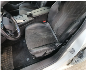
Seat Front Left / Bottom Coating / Replace-worn
