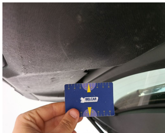
Trunk Lid Interior Coating / Complete Panel / Replace-scratch
