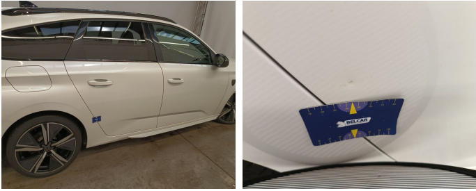
Door Rear Right // Repair & Painting-scratch + dent
