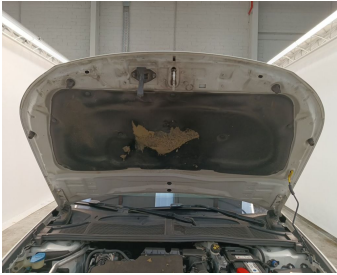
Front Bonnet / Insulation / Replace-tear
