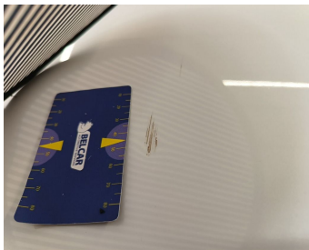
Front Bonnet // Repair & Painting-scratch + dent
