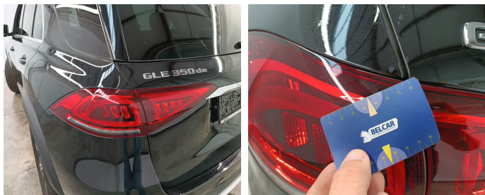
Light / Rear left / Replace-scratch
