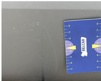
Bumper Rear / Spoiler / Replace-scratch
