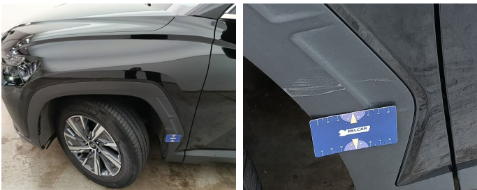
Wing Front Left / Trim / Replace-scratch
