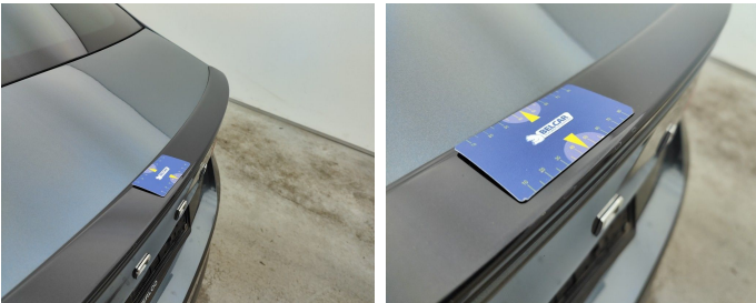
Rear Bonnet // Smart Repair Large-scratch
