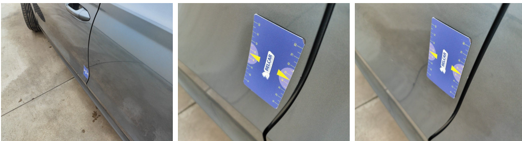
Damage within Renta-norm-
