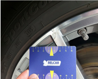
Wheel Two Tone Front Right // Repair-Chipped paint
