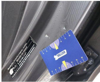
Rocker Panel Left // Smart Repair Medium-scratch + dent
