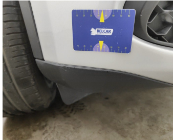
Bumper Front / Trim Right / Replace-scratch
