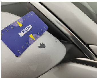
Central Console / Cover Armrest / Replace Cover Armrest-tear
