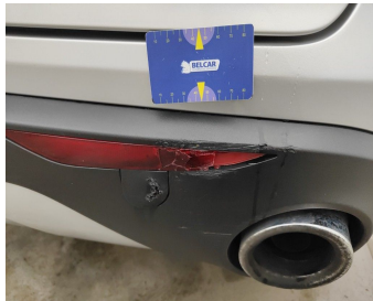
Back Side / Reflector R / Replace-cracked
