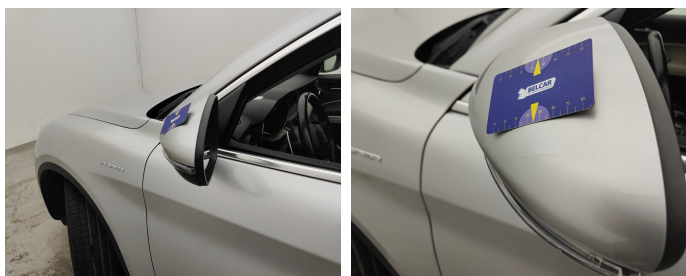
Side View Mirror Left // Polish-scratch
