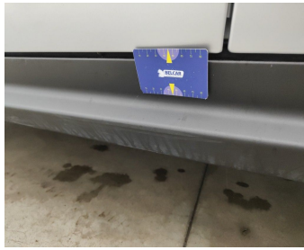
Rocker Panel Left / Cover Not Painted / Replace-scratch
