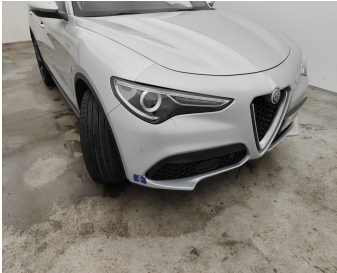
Bumper Front / Trim Right / Replace-scratch
