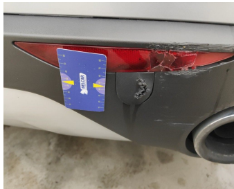
Towing Cover Rear // Replace-scratch
