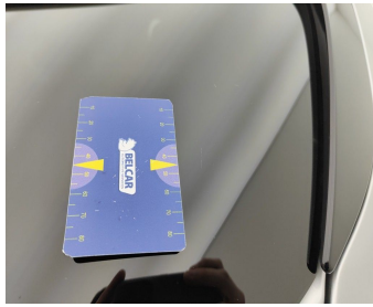
Rear Bonnet / Rear Window / Replace-scratch
