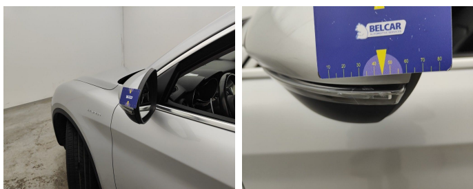
Side View Mirror Left / Direction Indicator / Replace-scratch
