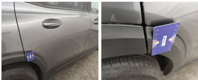
Door Rear Right / Trim / Replace-scratch
