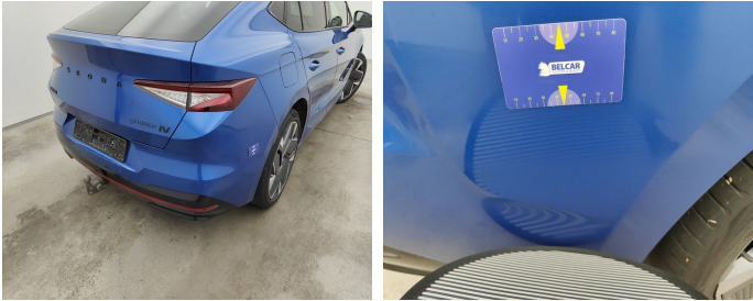
Bumper Rear // Painting-bad repair
