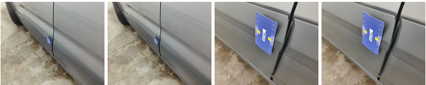
Door Front Left / Trim / Replace-scratch + dent
