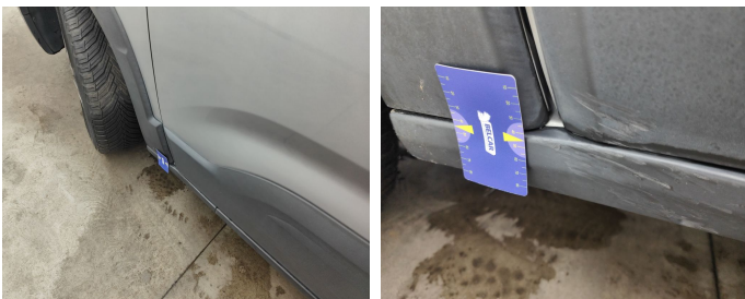
Door Front Left / Trim / Replace-scratch + dent
