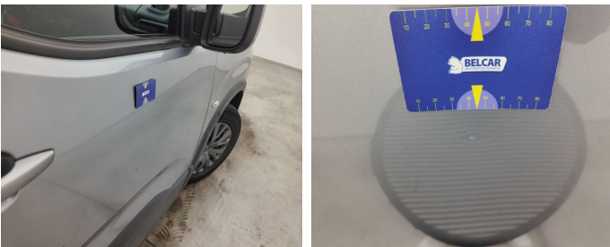
Door Front Right // Repair & Painting-scratch + dent
