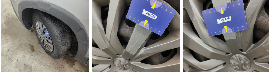
Wheel Front Left / Wheel Cover / Replace-scratch
