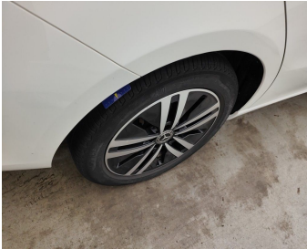
Tyre Rear Right // Replace-worn
