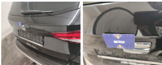
Rear Bonnet // Smart Repair Small-dent
