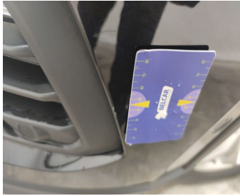
Bumper Rear / Spoiler / Replace-scratch
