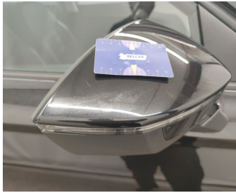
Side View Mirror Right // Polish-scratch
