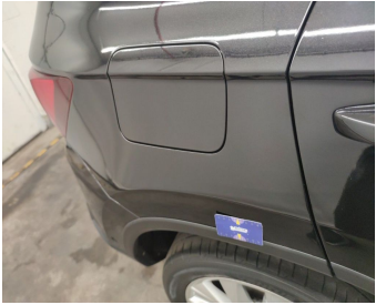
Wing Rear Right // Painting-bad repair
