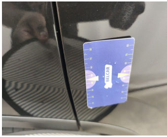
Door Rear Right // Painting-bad repair
